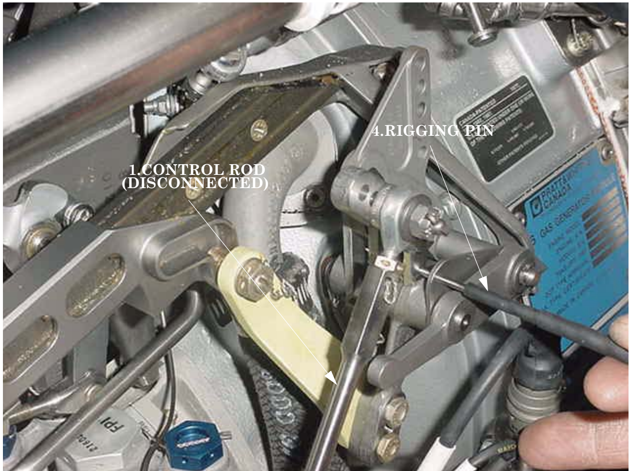
Fig. 214 - Fuel Control Unit (FCU) - Dead Band Adjustment (Sheet 2 of 6)
